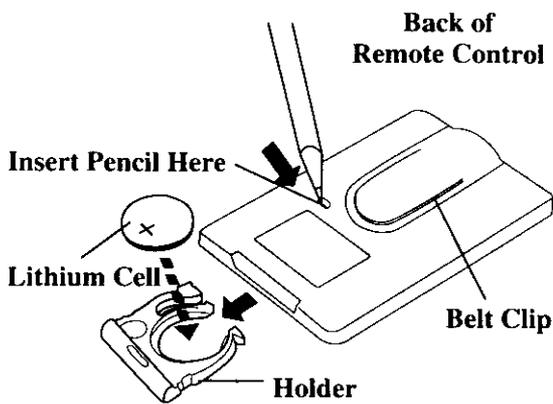
**Cautions:** Lithium cell battery. Replace only with 3-volt lithium cell – such as CR2025. Use of other cell presents a risk of fire or explosion. Must be disposed of properly. Never handle punctured or leaking cell. May cause burns or personal injury.
