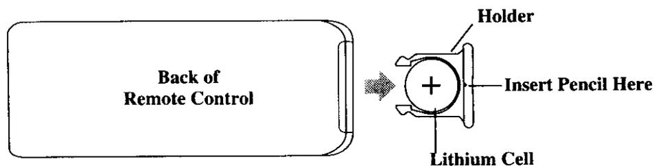
**Cautions:** Lithium cell battery. Replace only with 3-volt lithium cell – such as CR2025. Use of other cell presents a risk of fire or explosion. Must be disposed of properly. Never handle punctured or leaking cell. May cause burns or personal injury.
