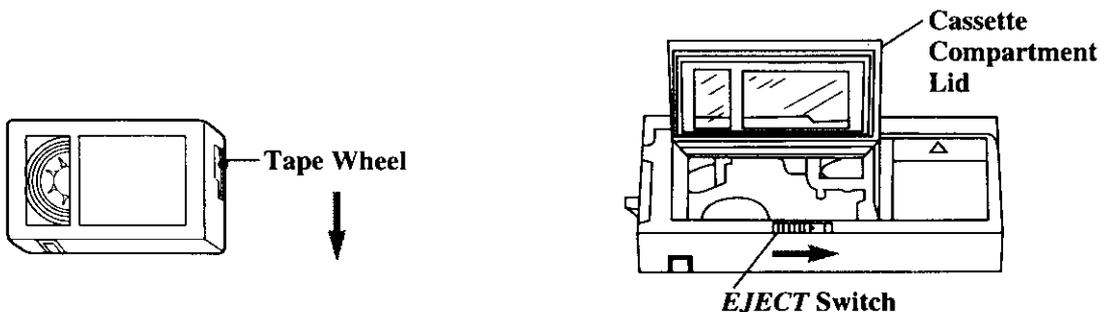
1. Before inserting the cassette into the adapter, remove any slack in the tape by turning the tape wheel on the side of the cassette.
