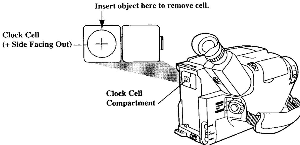
1. Make sure camcorder is turned off, and remove any power supply attached to the camcorder.
