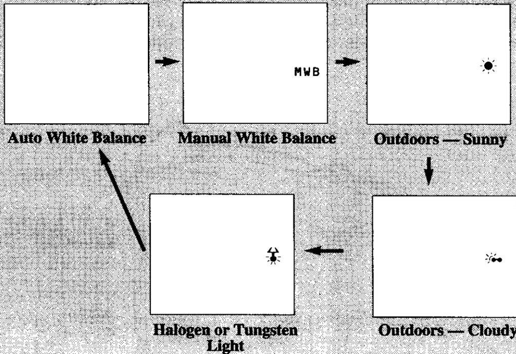
The *MWB* indicator will flash while the camcorder is adjusting white balance and stop flashing when it is ready to record.
