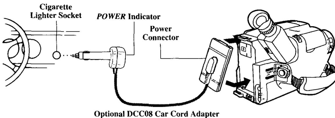
1. Place the *POWER* switch in *OFF* to turn off the camcorder. Power indicator on the camcorder turns off.
