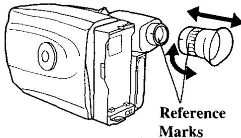
1. Turn the eyepiece counterclockwise and pull it out.
