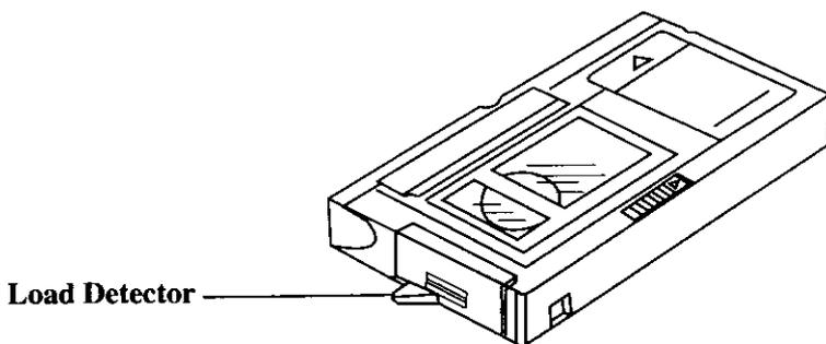
4. Gently close the cassette compartment lid until it locks into place. Make sure the cassette reel area under the adapter is free to turn while the cassette is loading.
