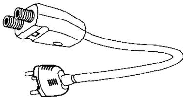
This RF output adapter is used with a coaxial RF cable, such as VH82 or VH90, to connect your camcorder to a standard TV (one without audio/video inputs) for playback. If your antenna cable is the flat twin-lead type attached by two screws, you will also need a 300-to-75 ohm transformer. If your TV has 300 ohm antenna screw terminals, you will need an optional 75-to-300 ohm transformer such as VH54.
