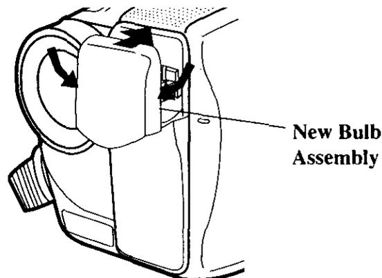
2. Place the the new bulb assembly into the camcorder *as shown*.
