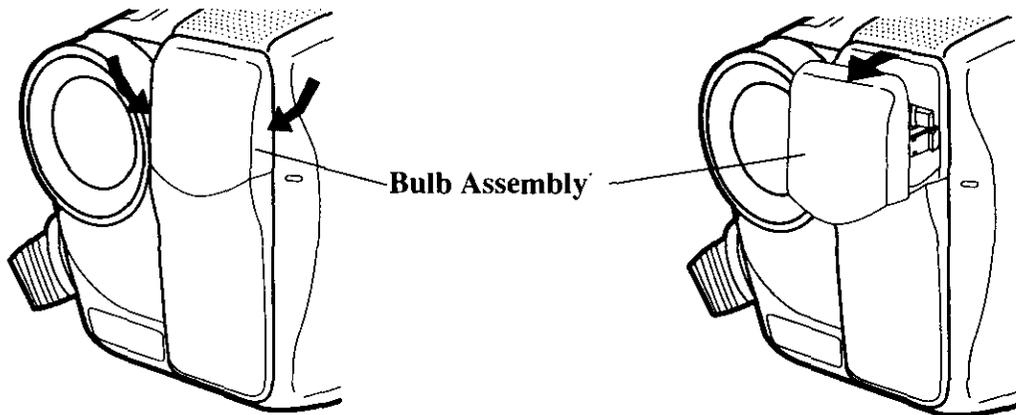
1. Pull on the sides of the bulb assembly and remove it from the camcorder *as shown*.
