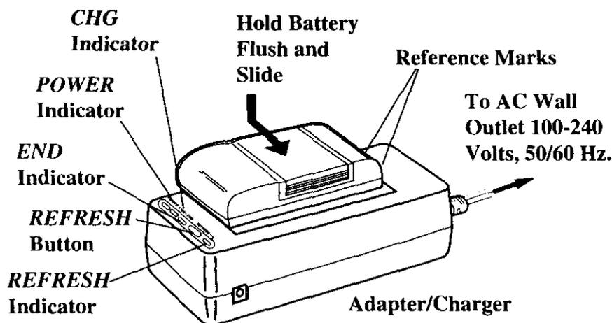
**Caution:** When a battery is attached to the adapter/charger, do not turn them upside down. The battery may fall off and be damaged or cause injury.
