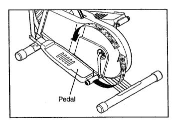
To dismount the elliptical glider, allow the pedals to come to a complete stop. CAUTION: The elliptical glider does not have a free wheel; the pedals will continue to move until the flywheel stops. When the pedals are stationary, step off the highest pedal first. Then, step off the lowest pedal.
