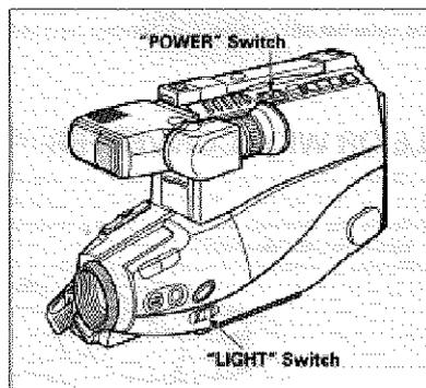
3. After use, set the **"LIGHT"** switch to **"OFF"** or set the **"POWER"** switch of the camera/recorder to **"OFF"** position.
