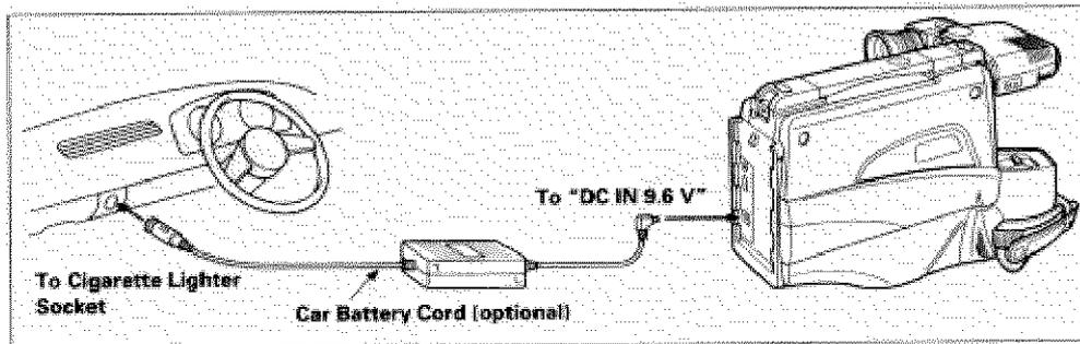
1. Connect the small plug of the car battery cord to the "DC IN 9.6V" jack of the camera/recorder.
