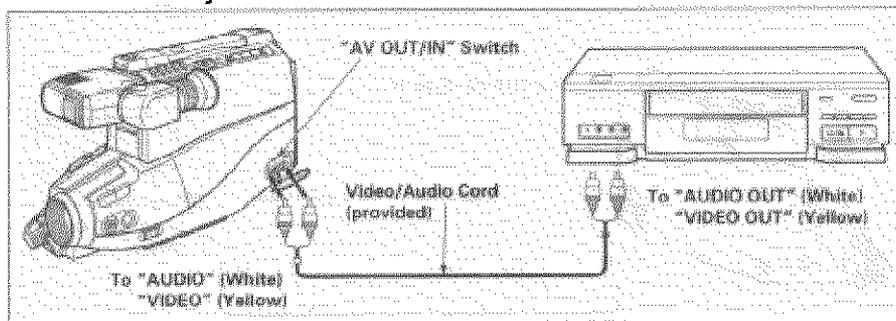
**NOTE:** When dubbing the sound and picture from a video source, set **"AV OUT/IN"** switch to **"IN"** position. When dubbing the sound and picture from the camera, set **"AV OUT/IN"** switch to **"OUT"** and do not connect **"AUDIO"** and **"VIDEO"** jacks.
