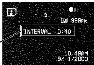
**6. Press the PHOTO button: Interval recording will start.**
