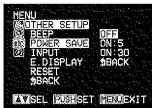
3. Turn the Select dial to change "OFF" to "ON:30" (power off in approximately 30 minutes) or "ON:5" (power off in approximately 5 minutes), and then press the Select dial.
