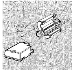
**3. Close the cover of core, taking care that it does not catch the DC power cable.**
