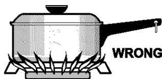
Never extend the flame beyond the outer edge of the utensil. A higher flame simply wastes heat and energy, and increases your risk of being burned by the flame.
