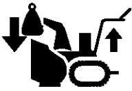
Weight Transfer Lift Handle To Engage
