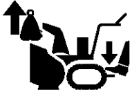
Weight Transfer Depress Pedal To Disengage
