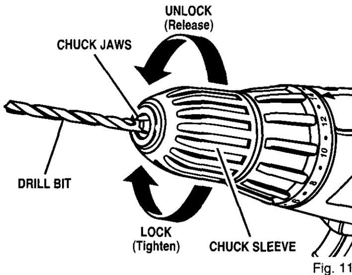
**⚠ WARNING:** Do not hold chuck sleeve with one hand and use power of the drill to tighten chuck jaws on drill bit. Chuck sleeve could slip in your hand or your hand could slip and come in contact with rotating drill bit. This could cause an accident resulting in serious personal injury.
