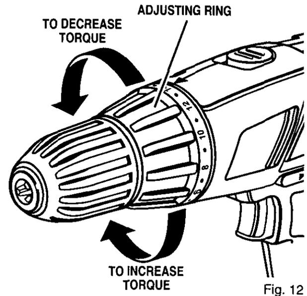
**Note:** Remember the two-speed feature (**HI-LO**) when setting torque. The amount of torque will vary depending on which speed setting you have your drill-driver. Switching to **LO** speed will increase torque. Switching to **HI** speed will decrease torque.
