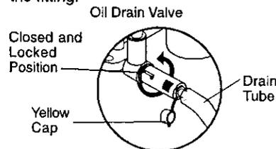
3. Unlock drain valve by pushing inward slightly and turning counterclockwise.
