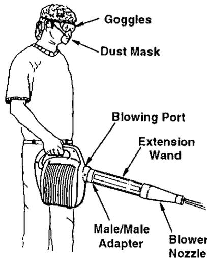
**WARNING:** Wear a dust mask if blowing creates dust which might be inhaled.
