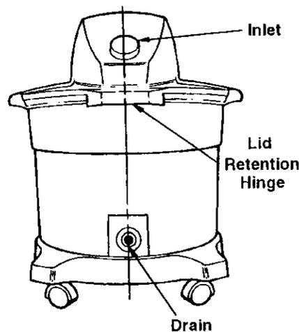
**NOTE:** For best appearance of the unit, the inlet of the vac should be located above the drain plug.
