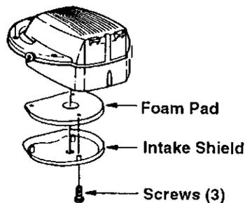
To clean the foam pad under the intake shield of the detachable blower:
