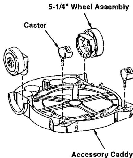
4. Position the dovetail portion of one of the wheel assemblies into the accessory caddy as illustrated. Tap the wheel support into the accessory caddy with a soft mallet. Repeat for the second wheel assembly.
