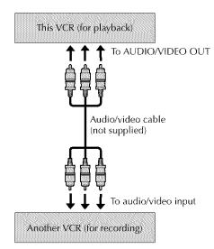
When using this VCR as the recording VCR, connect this VCR's audio/video input connectors to the audio/video output connectors on the other VCR. If the playback VCR is monaural, connect the audio output connector on the playback VCR to the left audio input connector on this VCR.
