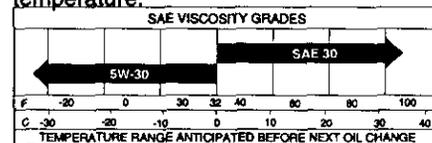
**NOTE:** Although multi-viscosity oils (5W30, 10W30 etc.) improve starting in cold weather, these multi-viscosity oils will result in increased oil consumption
