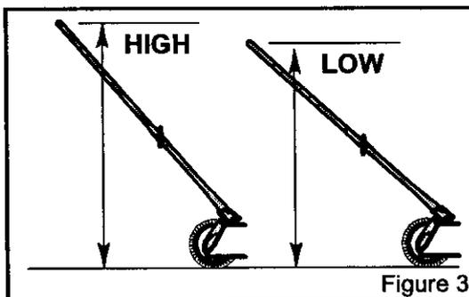
The **mounting holes** in the **lower handle** are offset (Figure 1). To change the hole offset, rotate the **lower handle**. This will change the
