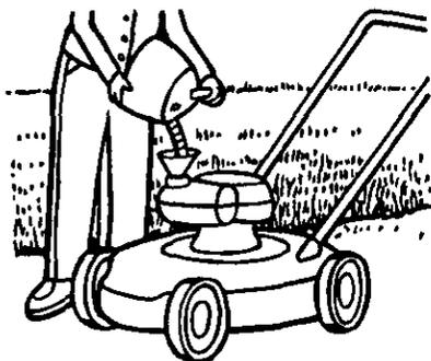
If you add gasoline to an engine that is running or hot, the result can be an explosion. Before you add gasoline, stop the engine and let the engine cool for several minutes. Remove dry grass and other debris from the mower. Keep the mower clean to improve the performance, help the engine and transmission run cooler, extend the life of moving parts, and decrease the danger of a fire.
