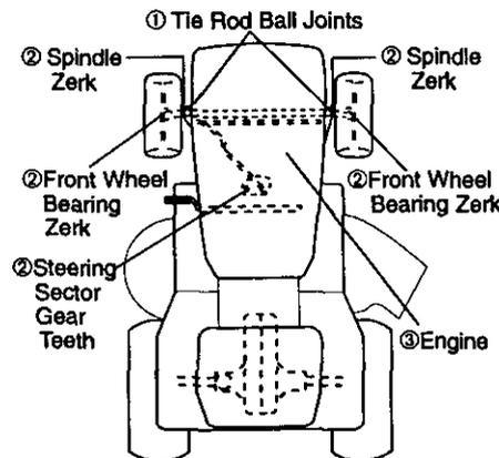
① Spray Silicone Lubriant (Move Boots to Lubricate)
