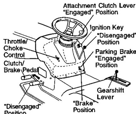
**IMPORTANT:** Leaving the ignition switch in any position other than "OFF" will cause the battery to be discharged, (dead).
