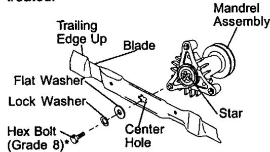
\*A Grade 8 Heat Treated Bolt Can Be Identified By Six Lines On The Bolt Head
