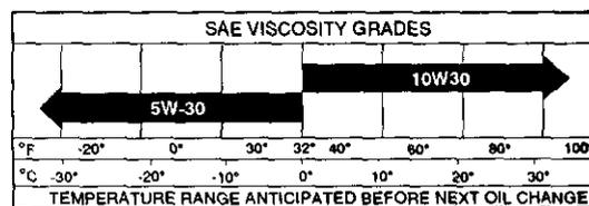
Change the oil after every 50 hours of operation or at least once a year if the tractor is not used for 50 hours in one year.
