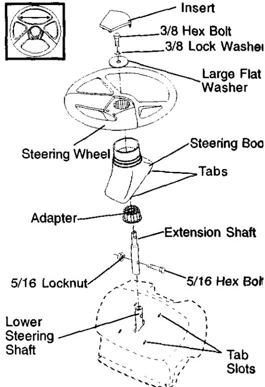
6. Assemble large flat washer, 3/8 lock washer, 3/8 hex bolt and tighten securely.
