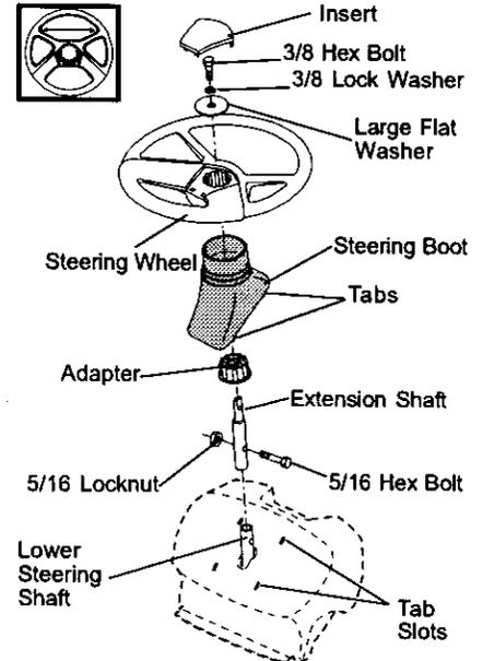
6. Assemble large flat washer, 3/8 lock washer, 3/8 hex bolt and tighten securely.
