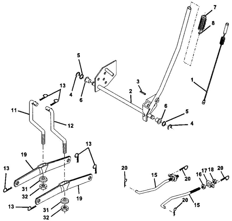
**LIFT ASSEMBLY      TRACTOR -- MODEL NUMBER 917.272065**
