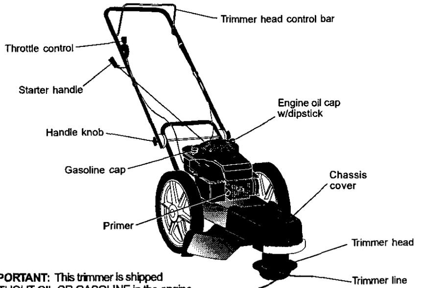
**IMPORTANT:** This trimmer is shipped WITHOUT OIL OR GASOLINE in the engine.
