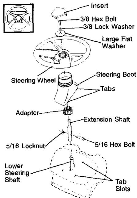
6. Assemble large flat washer, 3/8 lock washer, 3/8 hex bolt and tighten securely.
