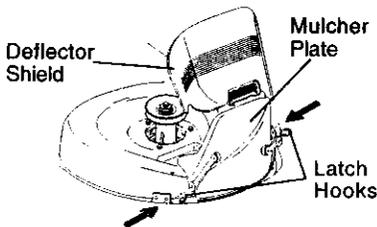
**CAUTION:** Do not remove deflector shield from mower. Raise and hold shield when attaching mulcher plate and allow it to rest on plate while in operation.
