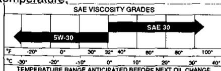
**NOTE:** Although multi-viscosity oils (5W30, 10W30 etc.) improve starting in cold weather, these multi-viscosity oils will result in increased oil consumption
