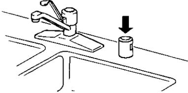
The drain air gap is usually located on top of the sink or countertop near the dishwasher. To order a drain air gap call 1-800-366-7278 and ask for Part Number 300096.
