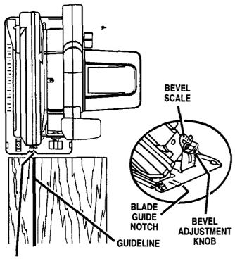
ALIGN INNER BLADE GUIDE NOTCH ON SAW BASE WITH LINE OF CUT AS SHOWN WHEN MAKING 45° BEVEL CUTS
