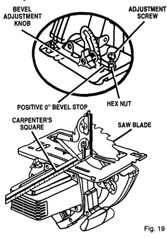
Your saw has a positive 0° bevel stop, that has been factory adjusted to assure 0° angle of your saw blade when making 90° cuts. However, misalignment can occur during shipping.
