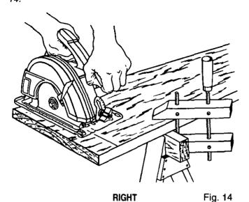
Squeeze the switch trigger to start your saw. Always let the blade reach full speed, then guide your saw into the workpiece.
