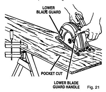
Squeeze the switch trigger to start your saw. Always let the blade reach full speed then slowly lower blade into the workpiece until base is flat against workpiece.
