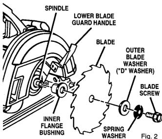
NOTE: Turn blade screw counterclockwise to remove.
