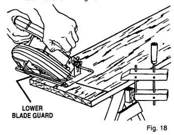
Rest the front edge of the base on the workpiece. Squeeze the switch trigger to start your saw. **Always** let the blade reach full speed, then guide your saw into the workpiece.
