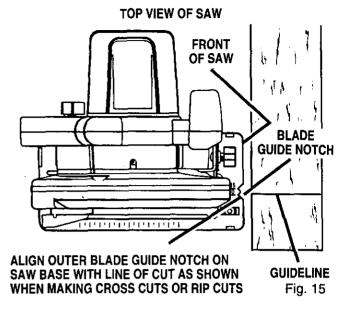
Since blade thicknesses vary, always make a trial cut in scrap material along a guideline to determine how much, if any, the guideline must be offset to produce an accurate cut. **NOTE:** The distance from the line of cut to the guideline is the amount you should offset the guideline.
