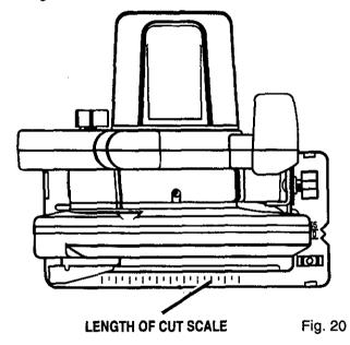
A length of cut scale has been provided on the base of your saw. It is parallel with the saw blade and can be used to measure the distance into material the blade has cut. **NOTE**: Six inches is the maximum length of cut that can be measured. Also, it is accurate only when the depth of cut is set at full maximum depth.
