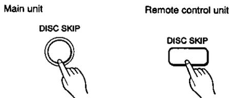
Each time the DISC SKIP button is pressed, the selected disc number changes from 1 to 5, then back to 1.
