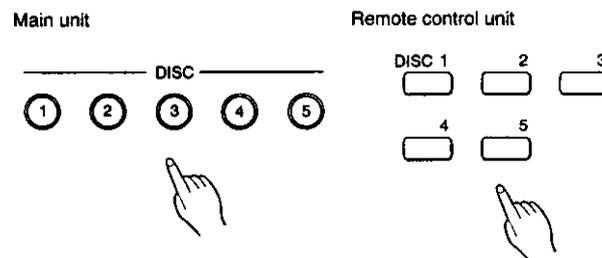
To select a disc, press the desired disc number (1-5). The unit searches for the selected disc and playback starts automatically.
