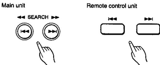
To skip back to the beginning of the track being played, tap the left button. When the beginning of the track is reached, tapping this button again skips to the previous track.
