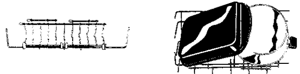
Flip away the entire row of both plate and bowl tines to make room for larger pans or roasters.
