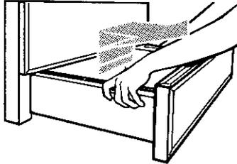
1. Empty drawer of any pots and pans before removing drawer. Pull drawer straight out to the first stop. Lift front and pull out to the second stop.
