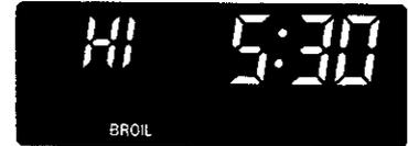
2. Press the TEMP (▼) keypad to lower the temperature in 5°F amounts. The broil range is 170°F - HI (525°F).
