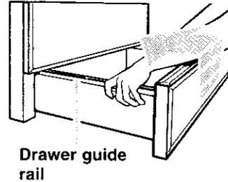
1. Position the drawer rollers under the rollers on the range. At the same time, fit the drawer guide rails on top of the rollers on the range.
