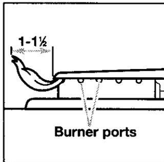
A good flame is blue in color not yellow. If the flames are not burning at all ports, you may need to clean the burner ports.
