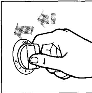
**NOTE:** All four electric ignitors will click at the same time. However, the burner with the control knob turned to LITE is the one that will ignite.
