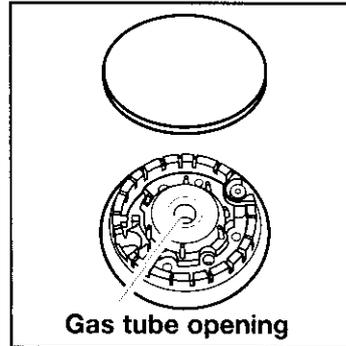
To replace the burner cap, make sure the alignment pins on the cap are properly aligned with the burner base.
