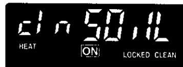
**3. After the SELECT CLEAN Self-Cleaning cycle ends: LOCKED goes off and the door unlocks.**
