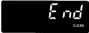
7. Press any pad to remove "End" and bring back time of day; or open door, at which time "door" will be displayed. Then close door and time of day will appear in display window.
