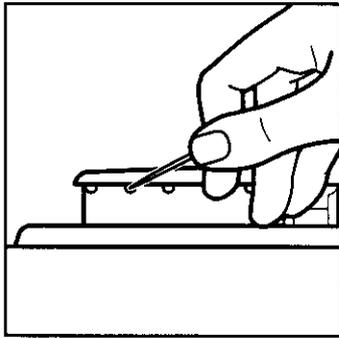
**Do not enlarge or distort the port. Do not use a wooden toothpick.** If the burner needs to be adjusted, call a qualified technician for service.
