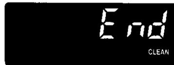
**4. Press any pad to remove "End" and bring back time of day; or open door, at which time "door" will be displayed. Then close door and time of day will appear in display window.**
