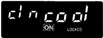
If the oven temperature is too high for you to immediately open the door when you press OFF/CANCEL, "cln," ON, "cool," and LOCKED will appear on the display until the oven cools; then "End" will appear and the door will unlock.
