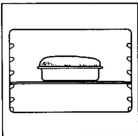
the preheat conditioning ends. During baking/roasting, the oven burner will turn on and off to keep the oven temperature at the setting.
