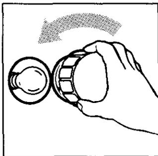
3. Remove the light bulb from its socket by turning it counterclockwise. Replace the bulb with a 40-watt appliance bulb.
