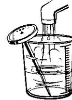
3. Check the temperature on the thermometer as the water is running into the cup.
