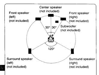
The front, center, and surround speakers should be placed at approximately the same distance from the listening position. The angles in the diagram are approximate.
