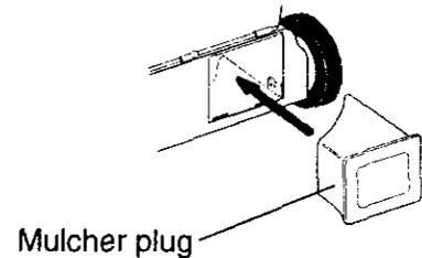
**CAUTION:** Do not run your lawn mower without mulcher plug in place or approved clipping deflector or grass catcher in place. Never attempt to operate the lawn mower with the rear door removed or propped open.
