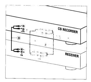
1 For playing back separately on the CD Player deck, connect a third cable ③ (not supplied) between the ANALOGUE OUT plugs on the CD Recorder and the INPUT plugs on an amplifier, e.g. CD or AUX.
