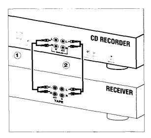
Use the audio cables supplied. Connect the red plugs to the R sockets, and the white plugs to the L sockets.
