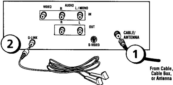
*PIP (Picture-In-Picture) won't work if you use this connection. You must connect a VCR to your TV with audio/video cables in order for PIP to work.*
