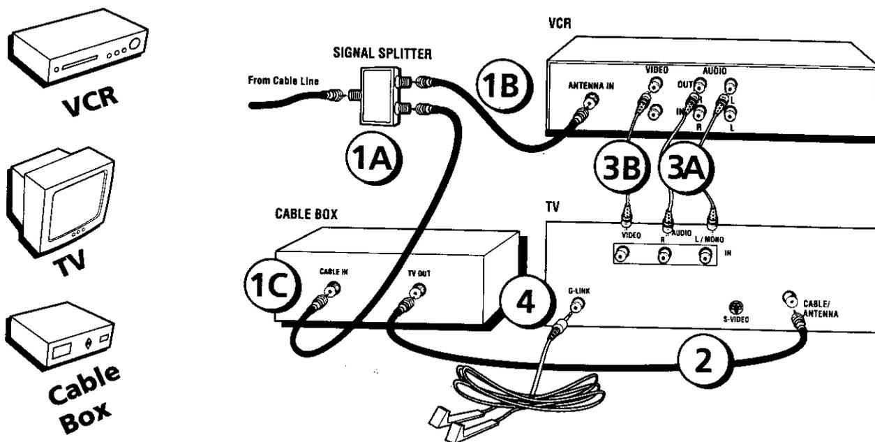
*Note: The GUIDE Plus+ system's One-Touch VCR Recording feature is not available with this connection. If you want to use the One-Touch VCR Recording feature with your cable box, you must use the TV and VCR connection on page 8. You can do so by routing the signal from your cable box into the antenna input on your VCR. Note that PIP won't work if you use this connection. This connection may not be compatible with all cable services, especially if some or all cable channels are scrambled.*
