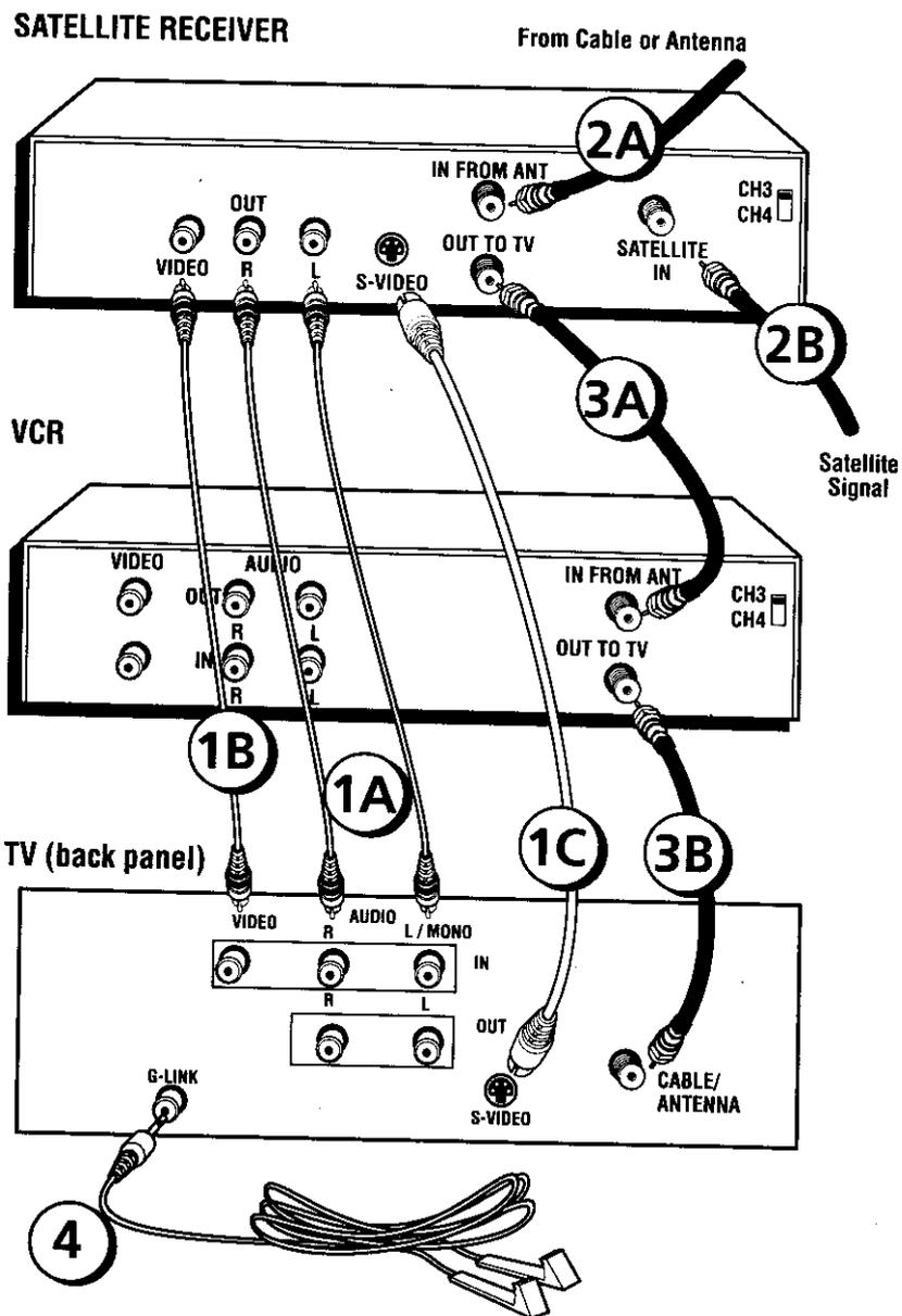
You need to connect your Satellite Receiver to your TV with audio/video cables (see picture above) in order for Picture-In-Picture (PIP) to work.
