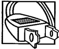
**Caution:** To prevent electric shock, match wide blade of plug to wide slot, fully insert.
