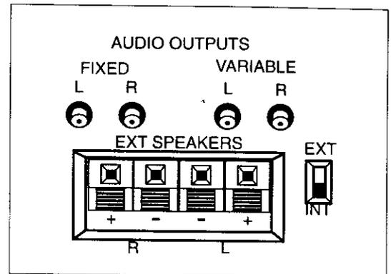
The **FIXED/VARIABLE OUT** jacks on the back panel provide a fixed or variable audio signal. When connected to "variable", they are ideal for use with an audio amplifier that does not have its own remote volume control. When connected to "fixed," the output volume stays the same no matter how the volume changes on the TV.
