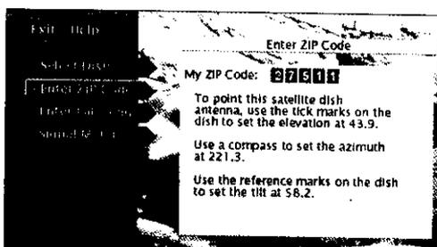
5. Record the elevation, azimuth, and tilt (oval satellite dish only) numbers below.
