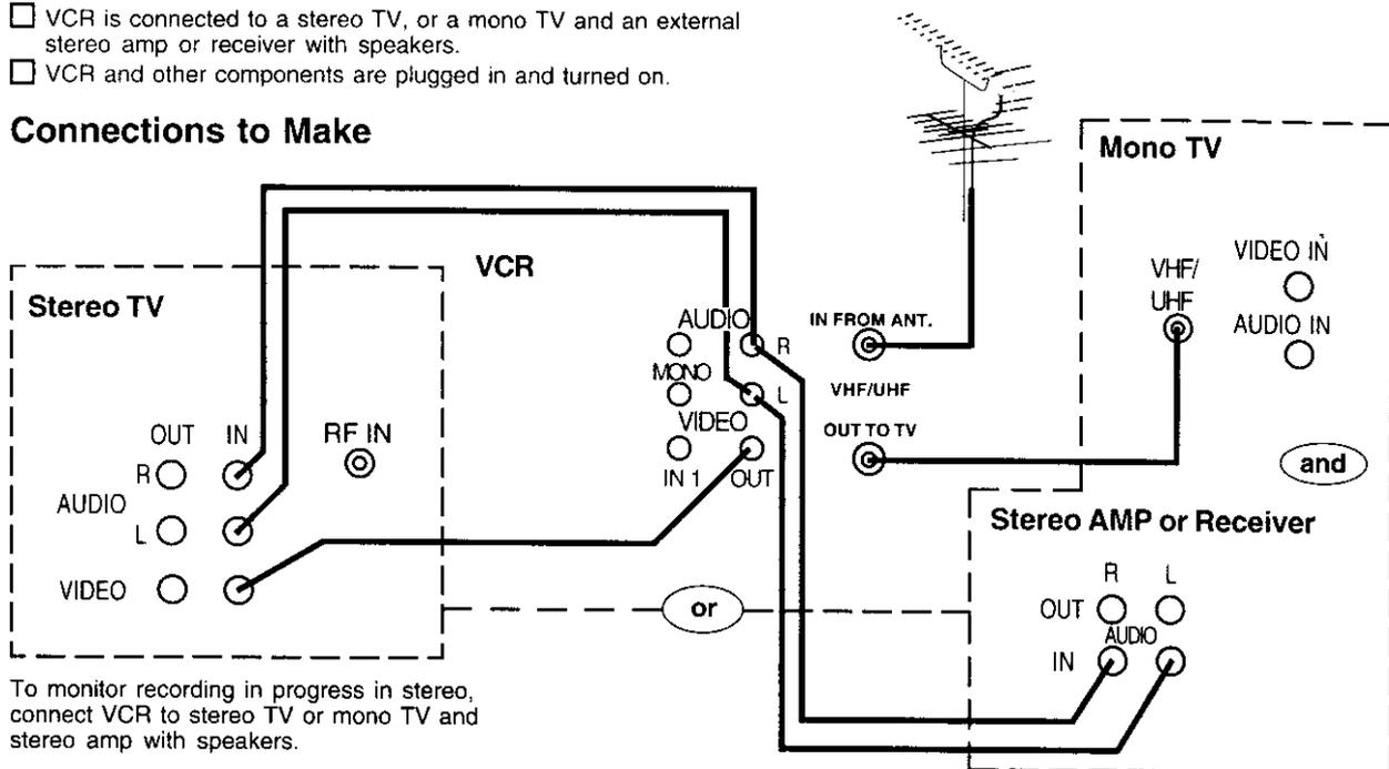
To monitor recording in progress in stereo, connect VCR to stereo TV or mono TV and stereo amp with speakers.
