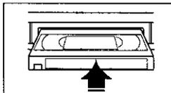
**Insert blank tape with record tab.**
