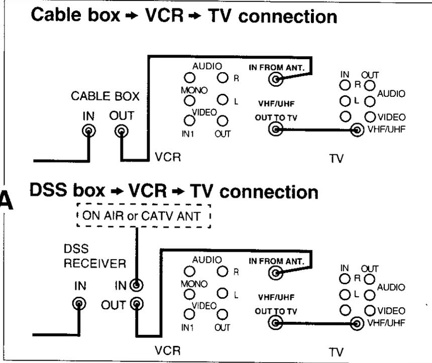
Note: You can not operate "Auto VCR Plus+ System Channel Setup" if type A connection is used.
