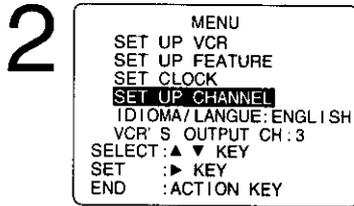
**Display SET UP CHANNEL.**
