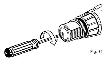
■ Insert allen wrench in chuck and tighten chuck jaws securely. Tap sharply with a mallet in a counterclockwise direction. This will loosen chuck on the spindle. It can now be unscrewed by hand. See Figure 15.
