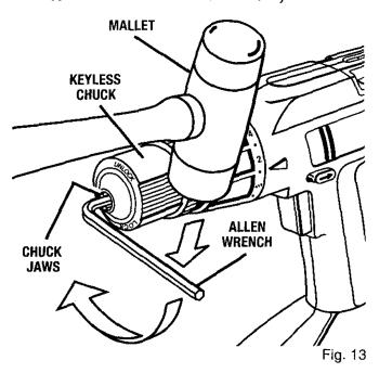
Open chuck jaws and remove allen wrench. Remove the chuck screw by turning it in a clockwise direction. See Figure 14. Note: The screw has left hand threads.
