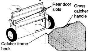
**ACAUTION:** Do not run your lawn mower without rear mulcher plug or approved grass catcher in place. Never attempt to operate the lawn mower with the rear door removed or propped open.
