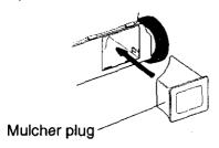
**ACAUTION:** Do not run your lawn mower without mulcher plug in place or approved clipping deflector or grass catcher in place. Never attempt to operate the lawn mower with the rear door removed or propped open.
