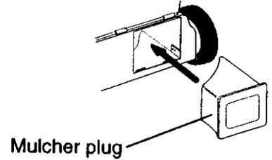
**CAUTION:** Do not run your lawn mower without mulcher plug in place or approved clipping deflector or grass catcher in place. Never attempt to operate the lawn mower with the rear door removed or propped open.
