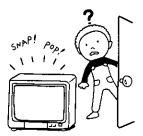
If a snapping or popping sound from a projection TV set is continuous or frequent while the projection TV is operating, unplug the projection TV and consult your dealer or service technician.
