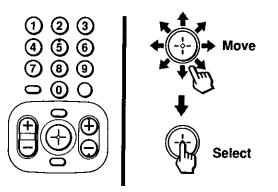
The supplied remote control has a joystick which moves the on-screen selector in eight directions. In most cases, moving the joystick up, down, left or right will cause the selector to move in the selected direction.
