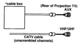
For this set up, you can switch between scrambled channels (through your cable box), and normal (CATV) channels by pressing ANT on your remote control.
