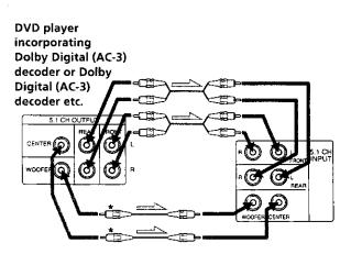
\* It is possible to use a pair of audio cords instead of two monaural audio cords to connect to the 5.1 CH INPUT CENTER and 5.1 CH INPUT WOOFER jacks.
