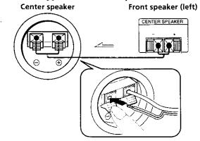
Be sure to connect matching speaker terminals (e.g., use the solid-color wire to connect + to +, and use the striped wire to connect - to -). If the connections are reversed (+ to -), the sound will lack bass.
