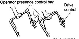
To engage drive control Drive control disengaged
