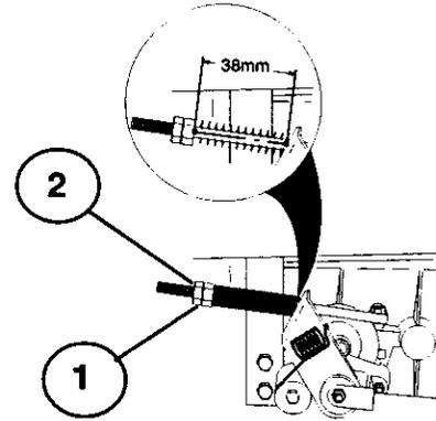
1. Measure the distance between the brake lever and the adjuster nut.
