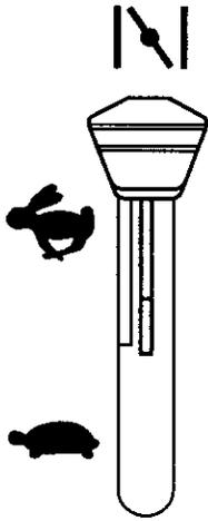
(Eng) Cold motor: Push the gas control up to end position choke (↑\↓)
