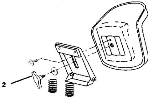
(Eng) Set the seat to the correct position by moving it forwards or backwards. Tighten the adjustment bolt securely (2).
