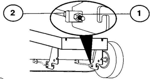
Eng To achieve best cutting results the cutting unit's front edge (B) should be about 10 mm (0.375") lower than the back edge (A). Adjust in the following way to raise the back edge:
