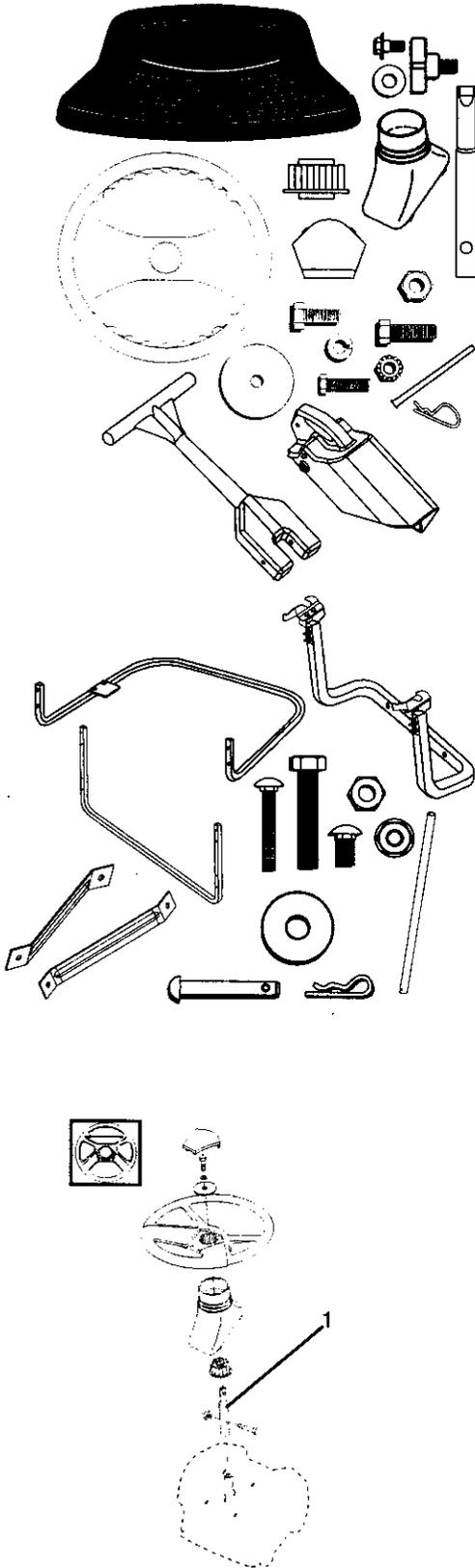
**Eng** Before the tractor can be used certain parts must be assembled, which for transportation reasons are enclosed in the packing. The picture shows which parts must be assembled.
