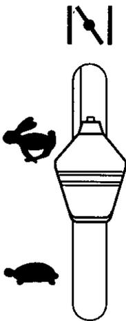
(Eng) Warm motor: Push the gas control half-way to full gas position "↔".
