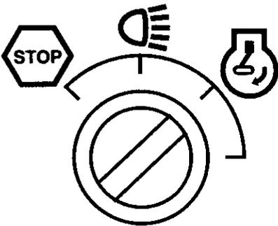
Ⓕ Let the ignition key return to the "ON" position when the engine has started. Push the gas control to the required speed. For cutting: full gas.
