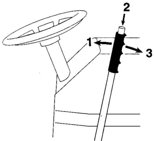
**Eng 6. Quick lifting/lowering of the cutting unit**
