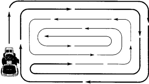
(Eng) Use the left side of the machine to cut close to trees, bushes and paths, etc. The blade cuts about 15 mm inside the edge of the cover.
