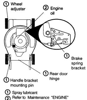
section. **IMPORTANT:** Do not oil or grease plastic wheel bearings. Viscous lubricants will attract dust and dirt that will shorten the life of the self lubricating bearings. If you feel they must be lubricated, use only a dry, powdered graphite
