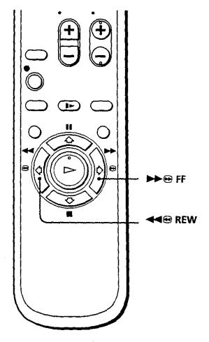
Hold down ▶▶ ⊕ FF (or ◀◀ ⊕ REW) for more than two seconds during stop. "SKIP" indicator appears on the TV screen.
