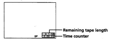
To check the remaining time of a T-140 or T-180 tape, set TAPE SELECT in the ADVANCED OPTIONS menu to 180. (For details, see page 85.)
