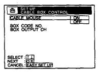
The TUNER PRESET menu appears. Set ANTENNA/CABLE to CABLE and press OK. For details, see page 50.
