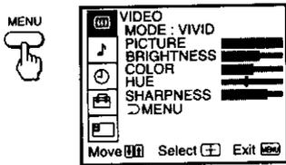
2 Press ▲ or ▼ to highlight the desired menu (in this case SET UP) and press (+) to select it.
