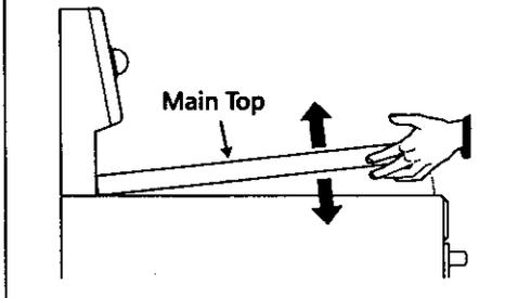
**⚠ WARNING** **DO NOT** turn the burners on when the cooktop is raised for cleaning. Be sure that the top is completely lowered and securely in place before turning on the burners.
