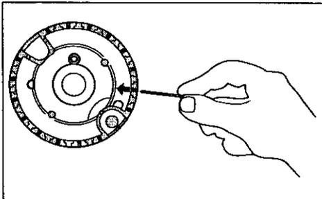
**CAUTION** Use caution when replacing the burner cap so the electrode is not damaged. This may cause a delayed ignition or prevent the burner from igniting.
