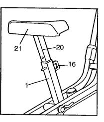
remove the Seat Pin (16). Align one of the holes in the Seat Post (20) with the hole in the Frame (1). Insert the Seat Pin into the Frame and the Seat Post. Caution: Make sure to insert the Seat Pin through one of the holes in the Seat Post; do not insert the Seat Pin under the Seat Post. In addition, make sure that the Seat Pin is inserted into the front of the Frame and the Seat Post as shown above.
