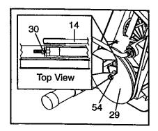
(29). To tighten the Belt, turn the Adjustment Nut (30) clockwise; to loosen the Belt, turn the Adjustment Nut counterclockwise. Make sure that the Flywheel is straight and tighten the Nylon Locknut (54). Reattach the side shields and pedals.
