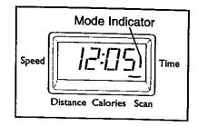
show that the scan mode is selected, and a flashing mode indicator will show which mode is currently displayed. Note: If a different mode is selected, you can select the scan mode again by repeatedly pressing the mode button. Speed, time, distance or calorie mode— To select one of these modes for continuous display, press the
