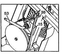
Strap, **fully** close the Strap Clamp. Turn the Crank (53) for a moment to make sure that there is not too much resistance. When the Resistance Strap is properly adjusted, reattach the left side shield and pedal.
