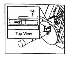
If the Drive Belt (14) is properly adjusted, reattach the side shields and pedals. If the Belt needs to be adjusted, loosen the Nylon Locknut (54) on the left side of the Flywheel
