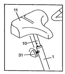
remove the Seat Pin (31). Align one of the holes in the Seat Post (10) with the hole in the Frame (1). Insert the Seat Pin into the Frame and the Seat Post. Caution: Make sure to insert the Seat Pin through one of the holes in the Seat Post; do not insert the Seat Pin under the Seat Post.
