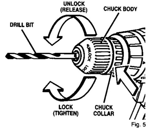
**WARNING:** Do not hold chuck body with one hand and use power of the drill to tighten chuck jaws on drill bits. Chuck body could slip in your hand or your hand could slip and come in contact with rotating drill bit. This could cause an accident resulting in serious personal injury.
